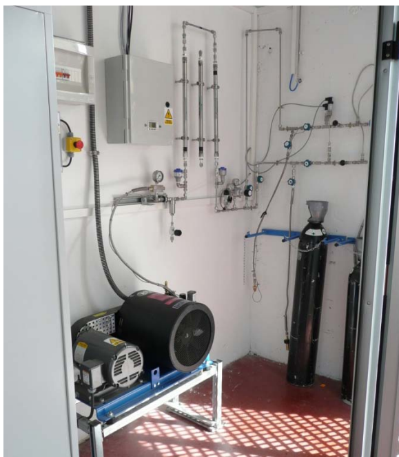
Fig. 8 : Picture showing the set-up for filling high-pressure cylinders using an oil-free RIX compressor.
