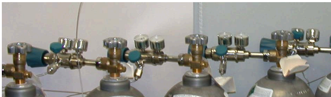
Fig. 7 : Picture showing Izaña N 2 O laboratory standards equipped with two-stage brass pressure regulators, manufacturer Scott Specialty.
