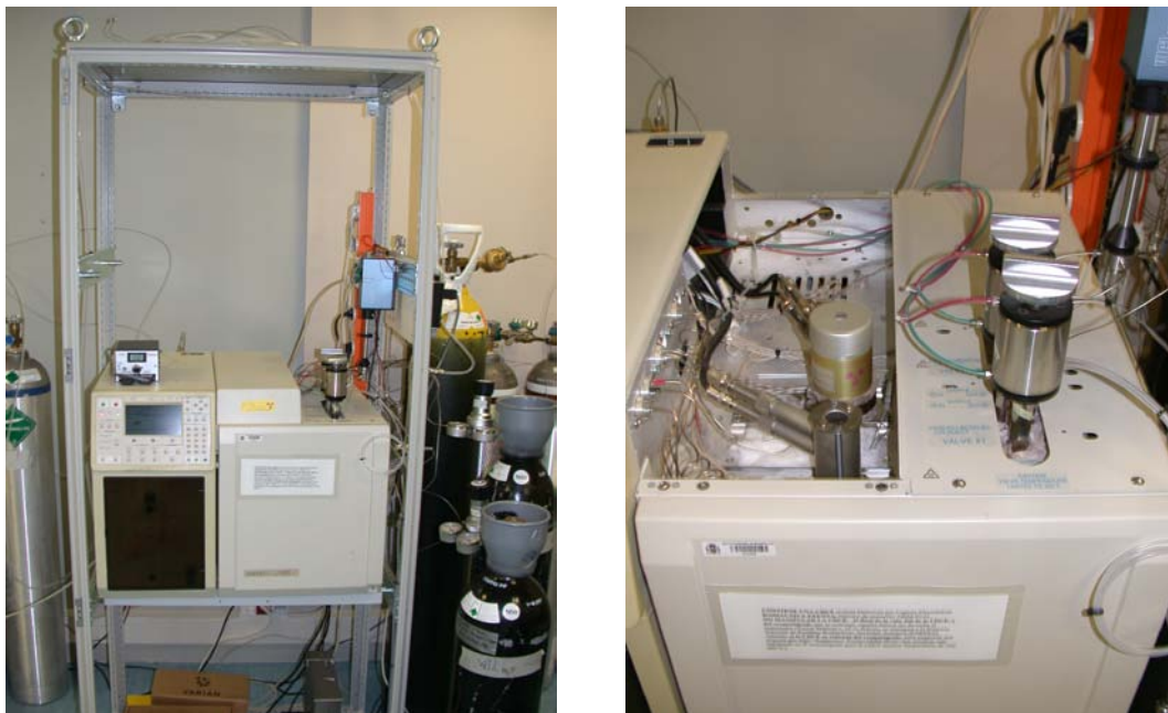
Fig. 6 : Pictures showing the N 2 O gas chromatographic system in the Izaña station laboratory.
