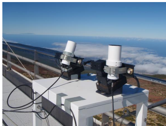
Figure 11.2. DOAS instruments outdoor optics with sky trackers.
