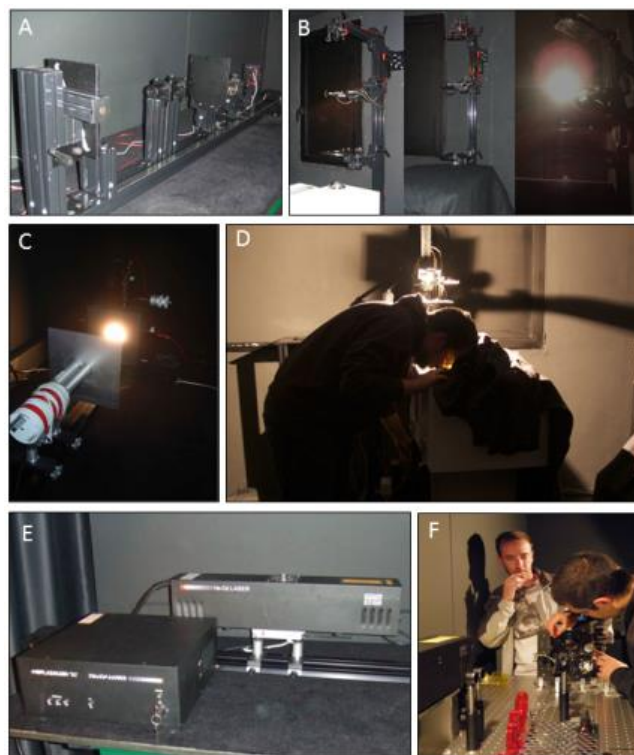
Figure 3.5. Images of the IZO Optical calibration facility. A) Horizontal absolute irradiance calibration set up, B) Three stages of a Brewer radiance calibration with the vertical set up, C) Absolute radiance calibration of a Cimel CE318, D) Angular response function determination of a Brewer (Photo: Alberto Redondas), E) Set up for Slit function determination and F) Alignment of a Brewer spectrophotometer optics (Photo: Alberto Redondas).
