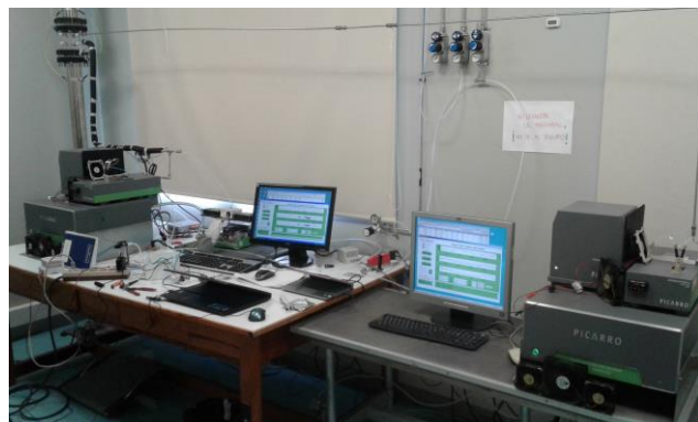
Figure 7.2. Intercomparison of the two Picarro L2120-I \delta D and \delta^{18}O analysers at the IARC.
