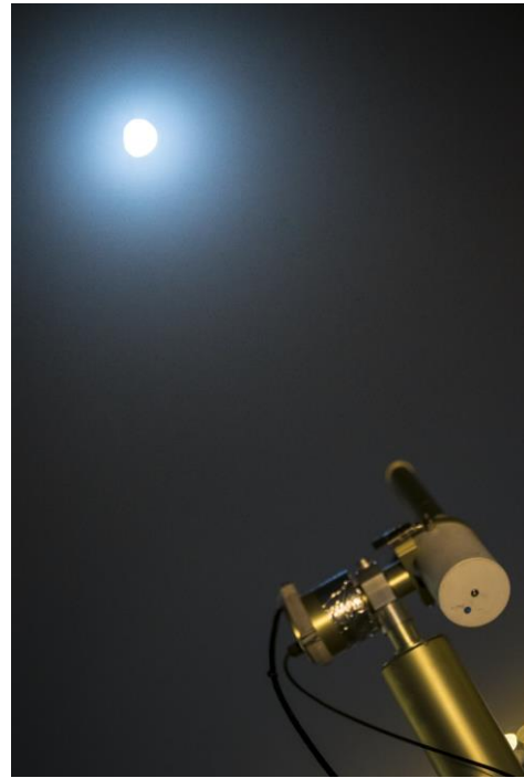
Figure 22.1. The CE318-T photometer tracking the moon at IZO.
