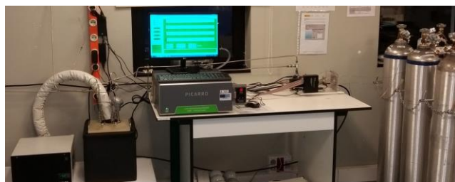
Figure 4.4. CRDS for measuring CO 2 , CH 4 and CO at the Izaña Atmospheric Observatory with the final plumbing design installed at the end of 2016.
