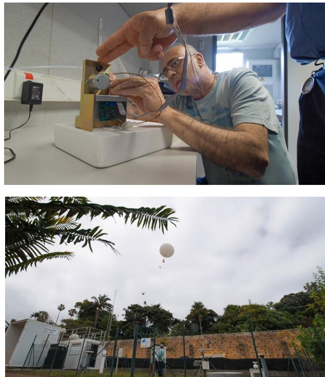
Figure 5.3. a) Preparation of an ozone electrochemical cell carried out by Sergio Afonso at the Ozonesonde Laboratory, BTO, b) launch of ozonesonde at BTO.
