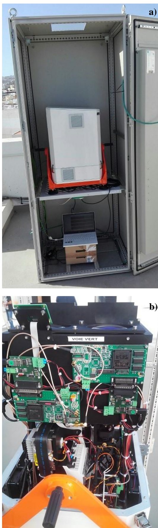
Figure 9.3 The new Cimel CE376 lidar: a) in the thermostated enclosure on the Santa Cruz Observatory instrument terrace and b) different details of the instrument.
