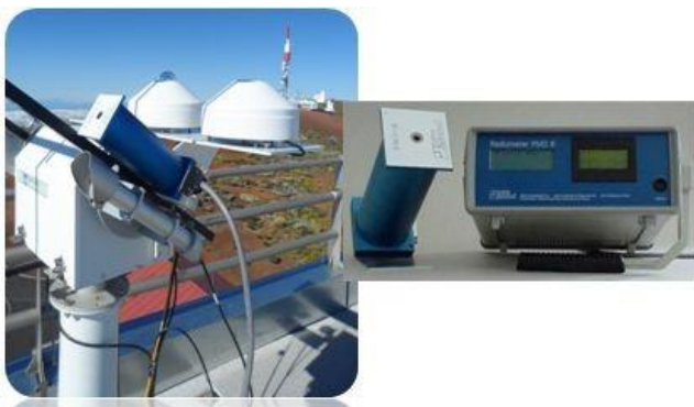
Figure 10.8. Absolute cavity radiometer (PMO6) installed at IZO during summers 2015 and 2016 in the BSRN sun-tracker.
