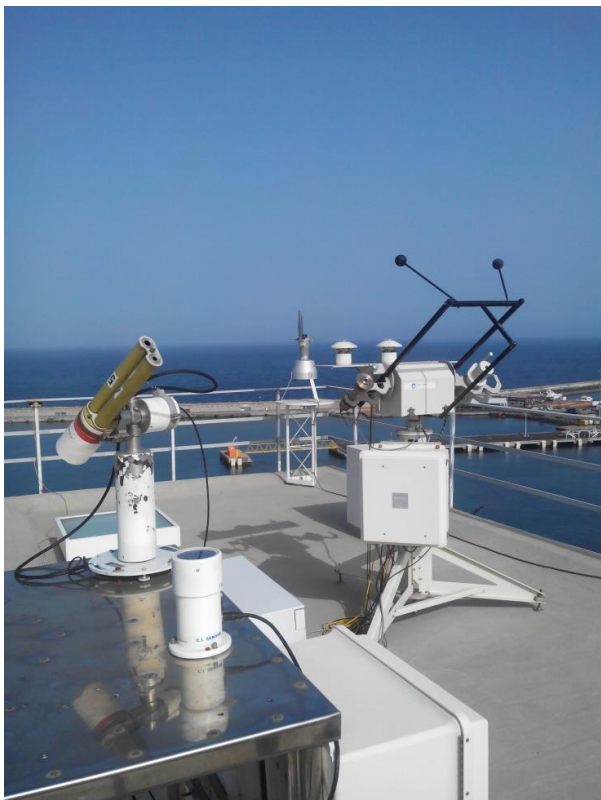
Figure 3.8. Image of Santa Cruz Observatory instrument terrace: ZEN-41-R radiometer (in the foreground), Cimel AERONET photometer, radiation instruments mounted on the sun-tracker and the HIRST pollen sampler (in the background).
