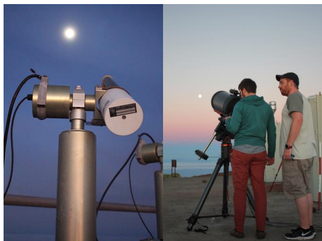
Figure 20.8. Instruments taking measurements of the moon during the 2017 lunar photometric field campaign (left: the Cimel CE318-T and right: the stellar photometers).
