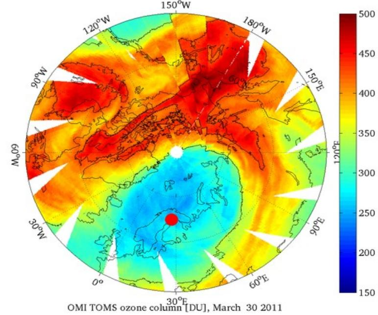
Left: Sodankylä sonde profiles from March 26 until March 31, 2011. They show ozone depletion in the vortex at around 20 km. Lowest values of ozone partial pressure in the soundings were around 3 mPa. Right: OMI TOMS total ozone on March 30, 2011. Red dot marks the location of Sodankylä station. OMI figure courtesy Janne Hakkarainen. Slide from Rigel Kivi, FMI-ARC.
