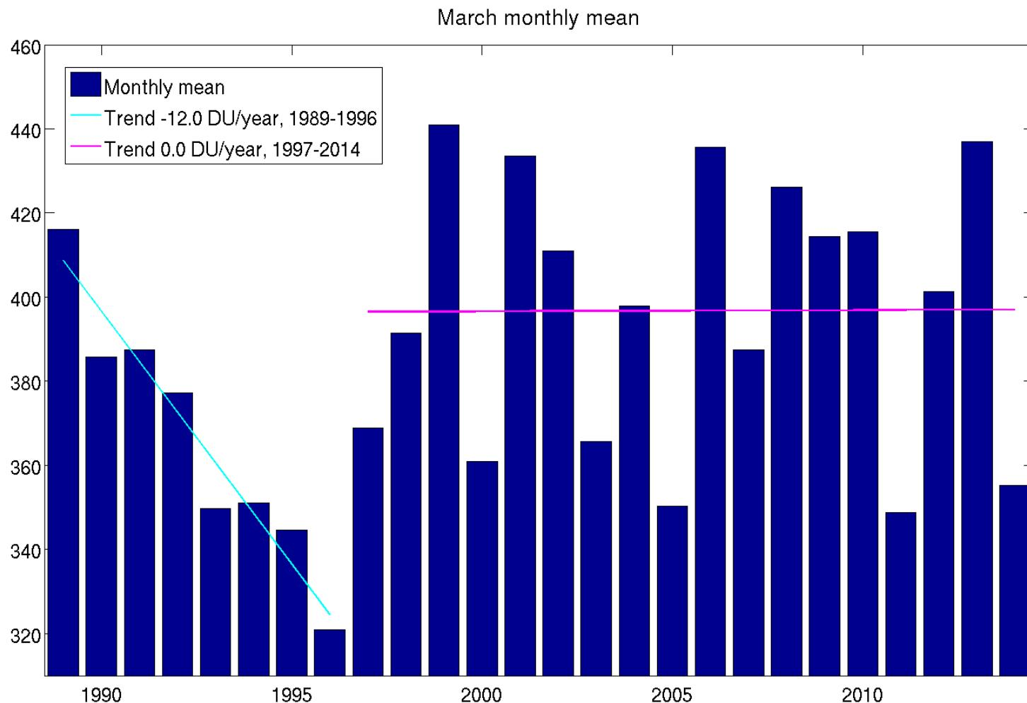
From Karppinen et al. 2016: Brewer spectrometer total ozone column measurements in Sodankylä Geosci. Instrum. Method. Data Syst. Discuss., doi:10.5194/gi-2015-41, 2016
