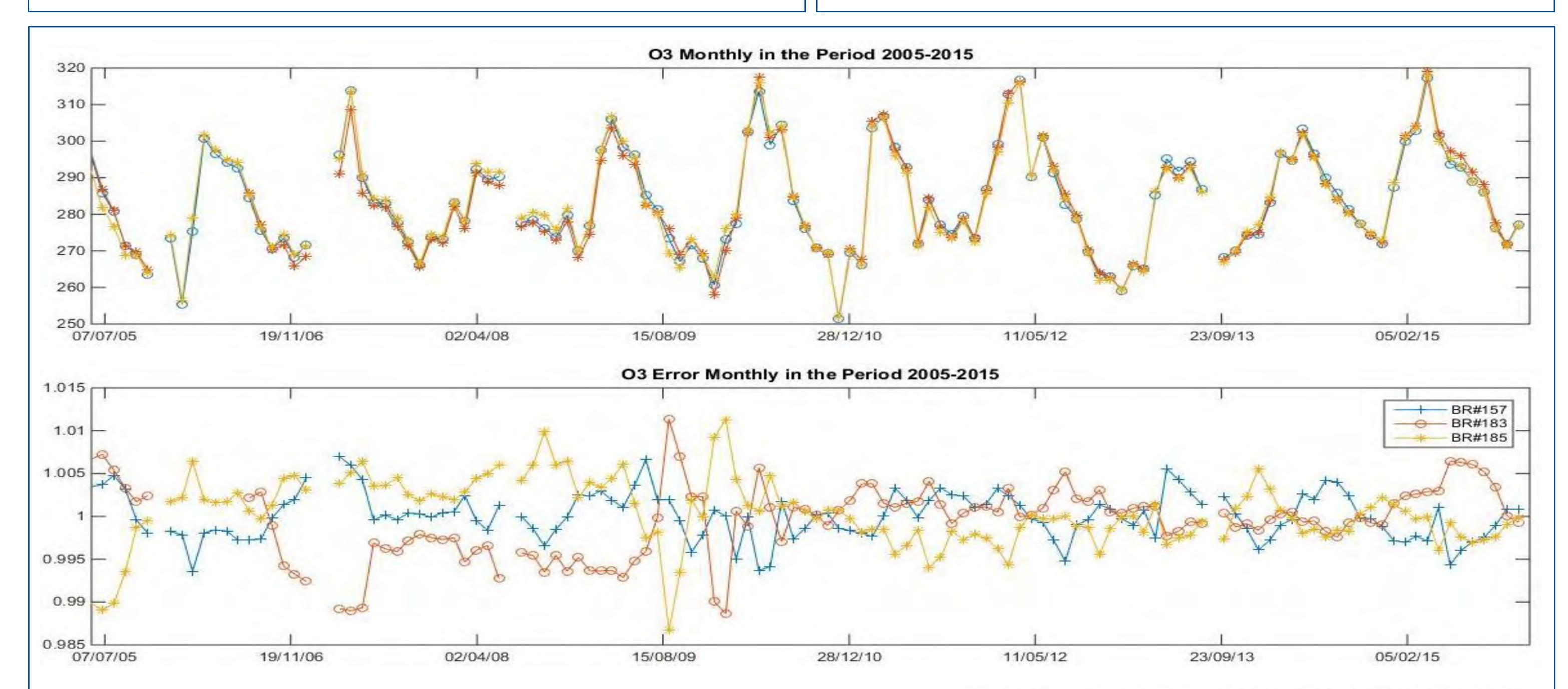
In the upper figure, the A coefficient obtained from the fit of the daily ozone measurements to  $2^{\rm nd}$  grade polynomial, as suggest Fioletov *at al.*[1] was monthly averaged for each Brewer. The ratio between the mean value of the three coefficient  $A_{\rm M}=(A_{157}+A_{183}+A_{185})/3$  and the particular coefficient of each Brewer can be used as a benchmark to estimate the performance of the instrument. As can be observed, the error is lower than 1% for the period 2005-2015.
