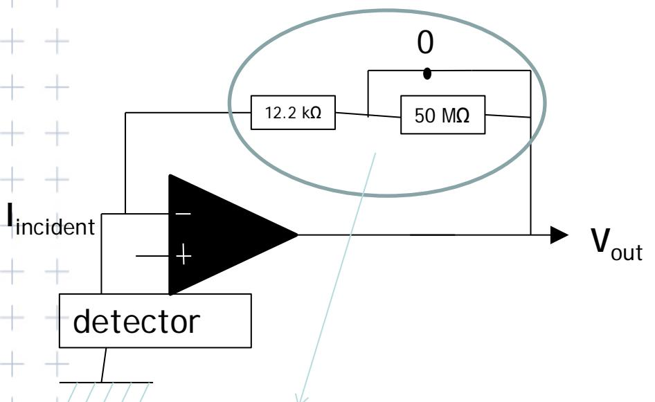
$$R_{eq} = \left[ \frac{1}{12.2\text{ k}\Omega} + \frac{1}{50\text{ M}\Omega} \right] = 12197.02\text{ }\Omega$$
